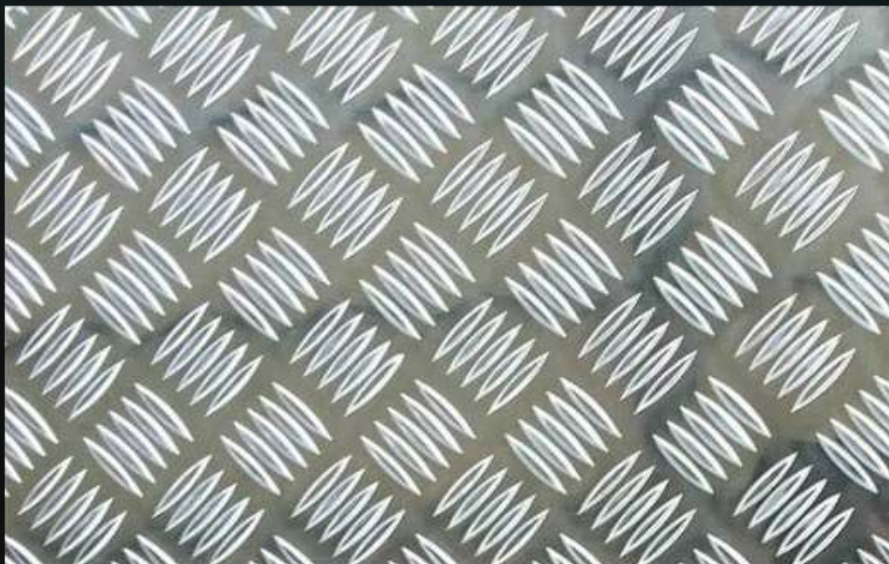
Arena floor material (aluminium checker plates)
